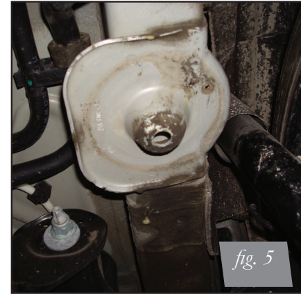
Previously Cut Spring Perch with Aftermarket Shock
