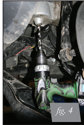
Previously Cut Spring Perch with Aftermarket Shock
