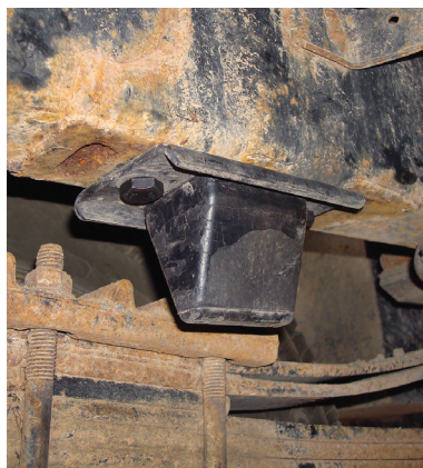
Most 2WD models have the jounce bumper bolted under the frame.
