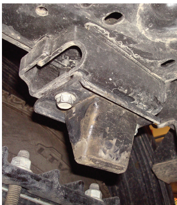
Most 4WD models have the jounce bumper bolted to a bracket.
