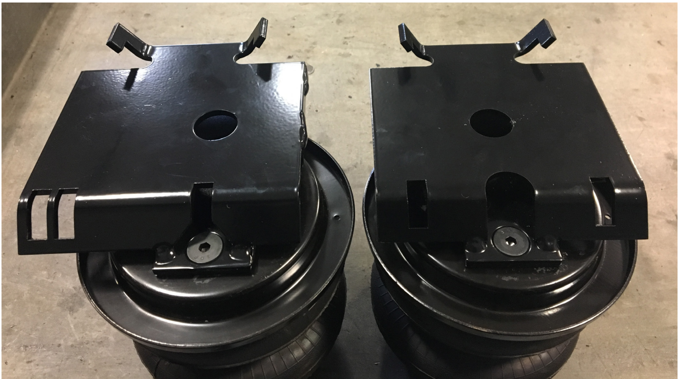
Left (driver's) side assembly using lower bracket (C1).
