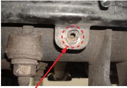
Fig. 22 File or die grind slots in the existing bracket holes to get the holes to line up enough to reinstall the screws
