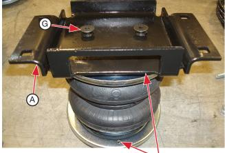
The window in the lower bracket must be on the same side as the fitting
