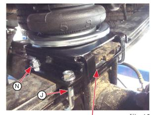
Window on lower bracket must be locked Fig. 15 around the tire side of the leaf spring retainer
