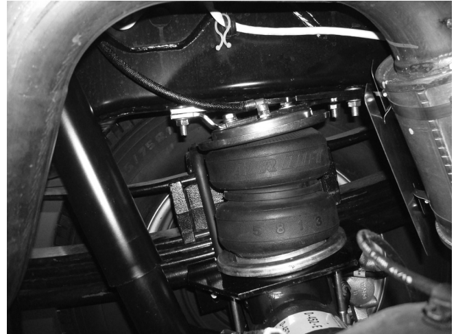
Inside, forward of axle view of passenger's (right) side installation.
