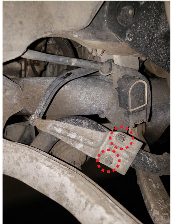
2. Disconnect the stabilizer bar linkage from the stabilizer bar.
