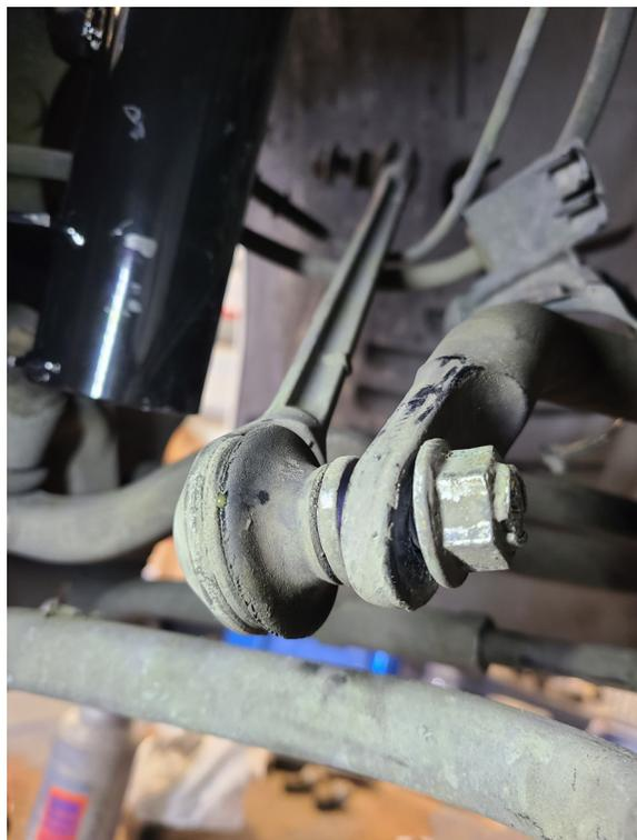
3. Clip the plastic tie holding the brake line bracket and slide the bracket out from behind the mount. To dislodge the bracket, use a flat blade between the plastic and the damper mount to unclip the plastic bracket from the mount and slide it out.
