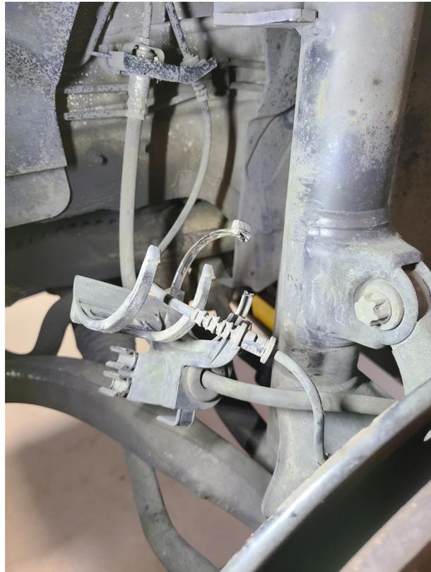
4. Unbolt the knuckle from the damper assembly.
