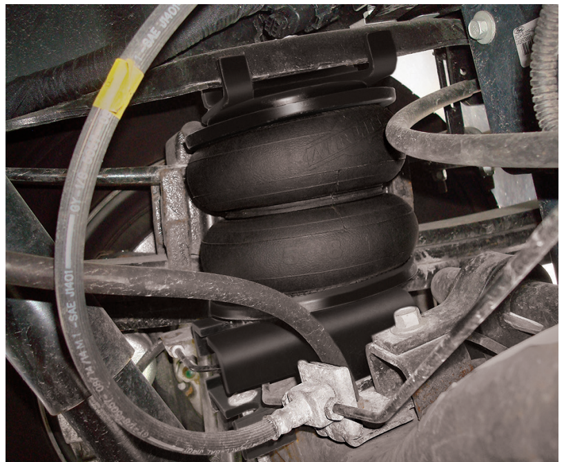
Inside view of the driver's (left) side installation.
