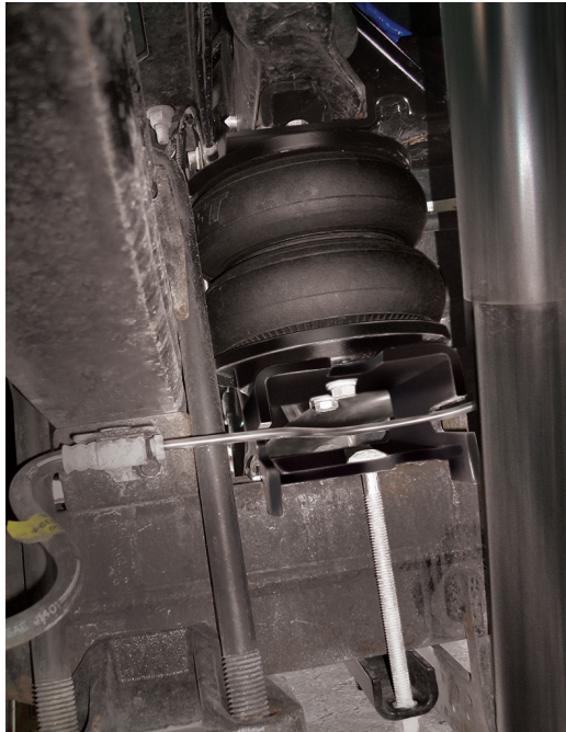
Rear view of driver's (left) side installation.
