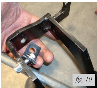
Attach the L-bracket to the brace in the position previously found using the hardware specified.
