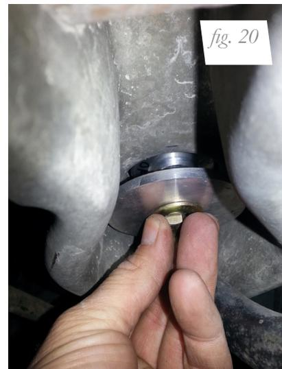
6. Remove the shock rod nut, upper washer and bushing from the new shock. Insert the shock into the shock tower, aligning the lower mount hole with the shock mounting bracket and insert the lower shock bolt through the mount (figs. 21-23). Do not torque at this time.
